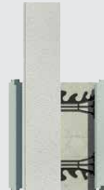
6" (150 mm) concrete core R-Value ratings based on exterior brick finish
