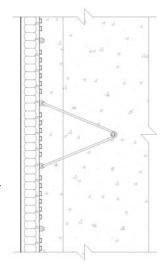
The new V-Clip will allow contractors even greater speed and flexibility when constructing multi-storey buildings with NUDURA. The V-Clip also reduces the need for additional bracing on the outside of the wall during concrete placement.
